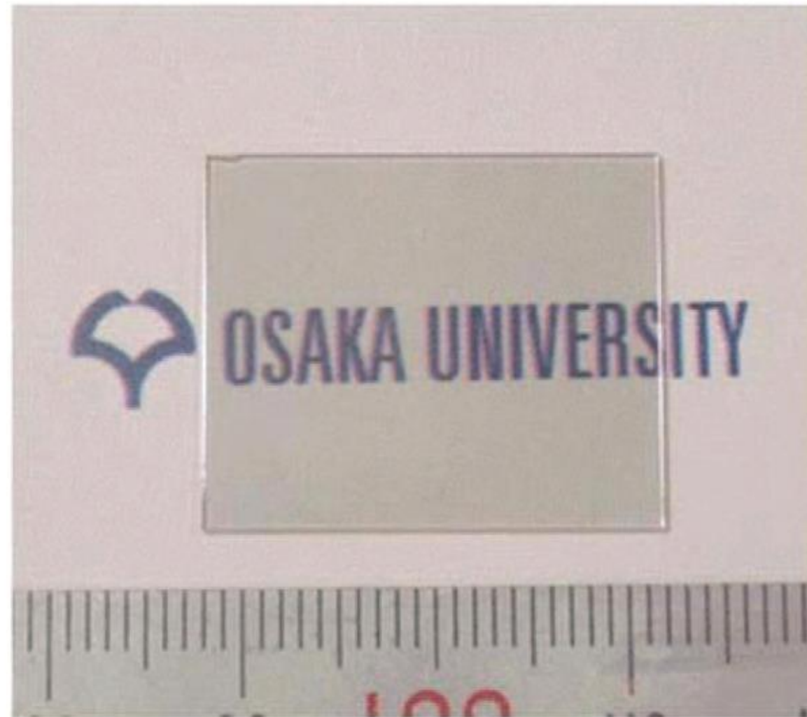
Figure 3. Photograph of the GaN crystal grown by Na flux LPE method on HVPE-GaN seed crystals. Both sides of the crystal were polished to the thickness of 750 \mu\text{m} to remove the seed crystals.
