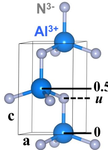
Instability of  $u$  in the transition region between ideal polar ( $u=0.375$ ) and non-polar ( $u=0.5$ ) structures leads to enhancement of  $\partial u / \partial \epsilon$ .
