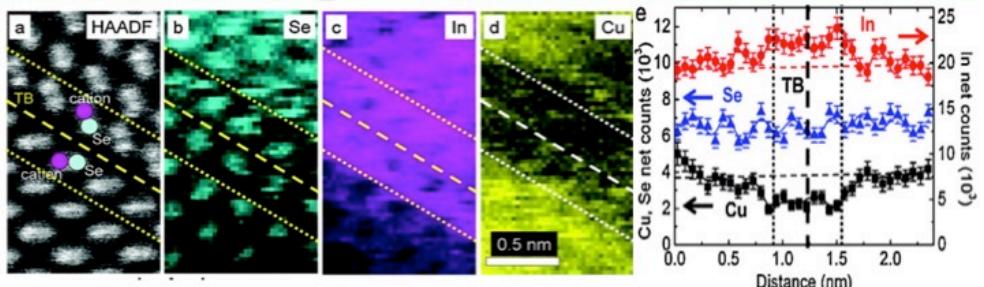
■ Spinodal Nano-decomposition : (Cu, V<sub>Cu</sub>), (Se, O), (In, Ga)
