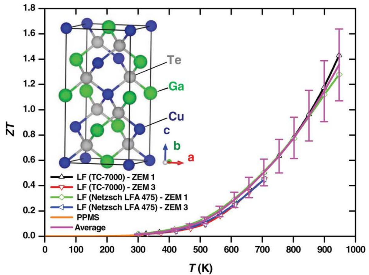
Figure 1. Temperature dependence of the dimensionless figure of merit  $ZT$  of polycrystalline bulk samples of CuGaTe<sub>2</sub>. The inset illustrates the crystal structure of CuGaTe<sub>2</sub>. Considering the uncertainty in the measurements of electrical resistivity, Seebeck coefficient, and thermal diffusivity, the error bars are a maximum of 21% for  $ZT$ .
