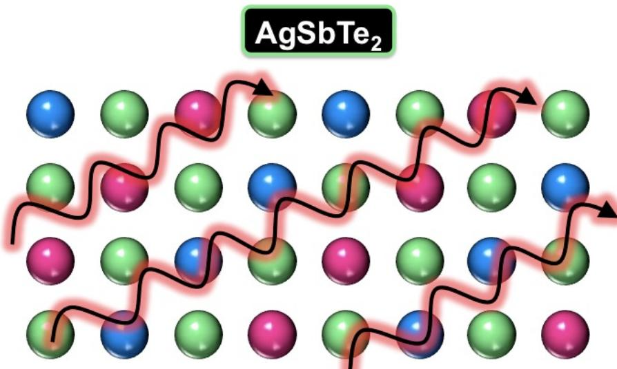
In Ag-poor condition,  $\kappa_L$  is small
